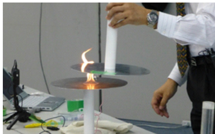
Lectures on static electricity: The basics of static electricity are studied through lectures incorporating experiments. (Shown here is an experiment involving an organic solvent catching fire due to static electricity.)
